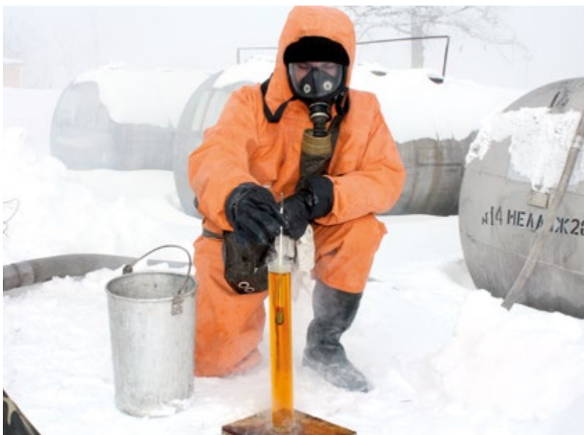
A member of the Ukrainian military takes a sample of the toxic rocket fuel component Mélange at the depot in Radekhiv, Ivano-Frankivsk region of Ukraine, before it is shipped for disposal. (OSCE/Leonid Kalashnyk)
